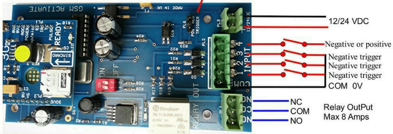
Input 4 only can be negative or positive triggerd (fig 1)
