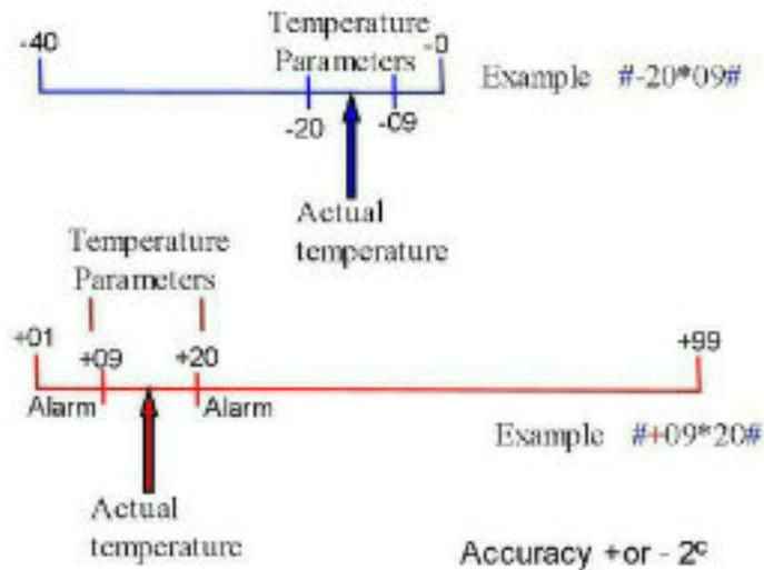
The Microprocessor will scan the temperature parameters every 3 minutes. When the temperature goes outside of the temperature parameters this will generate a text alarm sent to the users indicating the current temperature. When the temperature returns into the temperature parameters, a text will be generated to let users know temperature is normal
