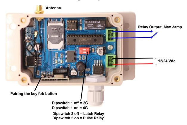
To pair the key fob to the GSM Smart Switch you will need to go through a process so that the key fobs are matched to the RF receiver on the GSM Switch
