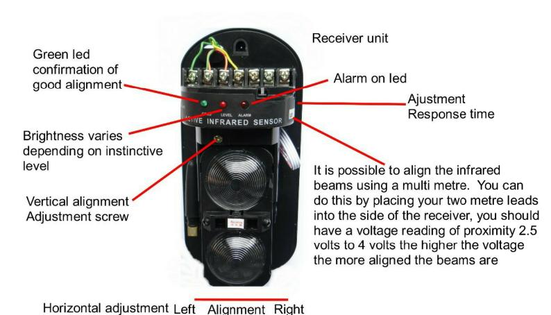
The voltage adjustment is only available on the receiver unit
